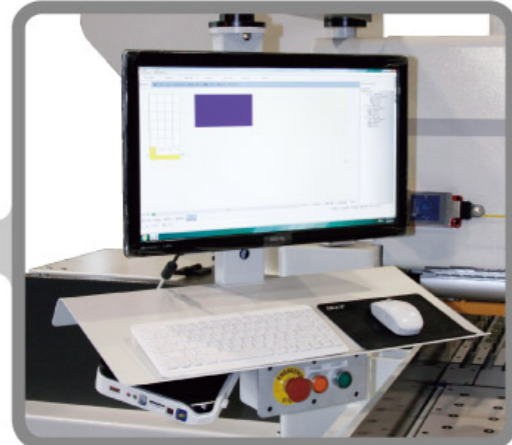
Option: PC_base, include optimizer software package. 選配：PC界面，提供優化排板選項。
