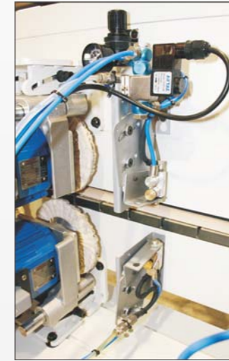
20. Cleaning agent spray system 清潔劑系統
