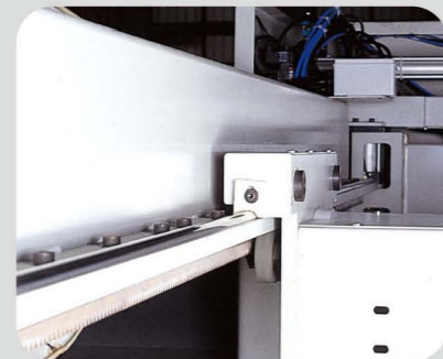
Hardened rail and heavy duty rack-pinion system.
