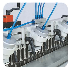
Angular cylinder clamp, assure the clamping direction and clamping force. 角度缸提供雙向壓著力，可確保加工基準線正確。
