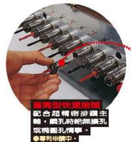
Cylinder type quick chuck.
