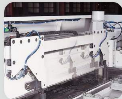
Independent side press roller system, automatic align the cross cutting at right angle.
