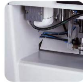
•Slope for dust collect 斜坡輔助集塵
