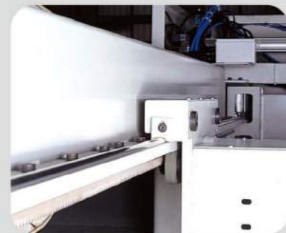
Hardened rail and heavy duty rack-pinion system.
