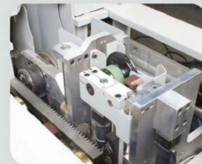
Remote adjustment device for scoring saw. (option)
