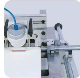
Stopper for top panel's checking point. 球面靠點確保參考點正確。
