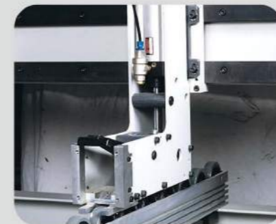
Extra size floating gripper with close-loop clamping force sensor.
