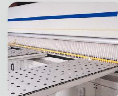
Floating table, modular bakelite working table and precision roller table.
